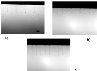
Figure 2. a) In-flight droplet image of a standard red LEP solution. b) Drop formation observed following adjustment of ink rheology. c) Final drop formation following optimization of drive conditions.
